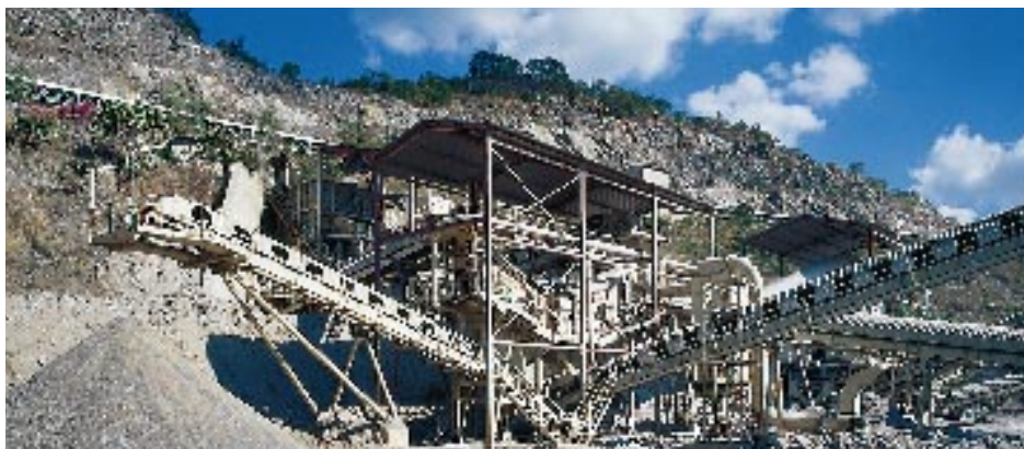
Nordberg has specialized in the turnkey design and delivery of complete crushing facilities. This turnkey facility was delivered to Siam Cement in southern Thailand. It is the company's largest cement plant and processes 300 tons of material per hour.
