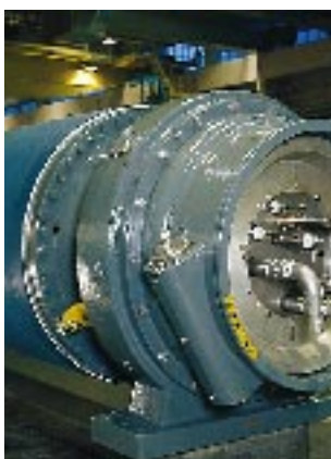
Powder metallurgically produced sleeve for paper machine presser suction roll represents innovative business developed by Rauma Materials Technology Oy.
