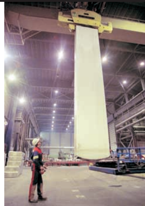
Rolling slabs up to 32 tonnes are cast at Elkem Aluminium Mosjøen for rolling mills in Europe.
