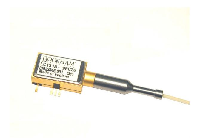
Bookham Technology's directly modulated 1310nm DFB laser combines ultrawide bandwidth with very high linearity over the wide temperature range of 25°C – 85°C, and represents a breakthrough for the realisation of the direct transport of analogue microwave/RF signals over fibre for inbuilding distributed antenna systems in cellular networks and for the burgeoning market in wireless LANs.
