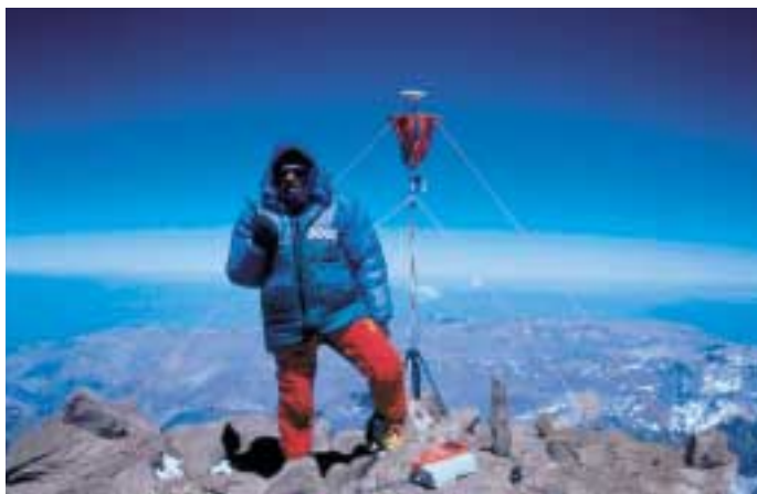
In January 2001 Mt.Aconcagua was remeasured. The highest peak of the Americas is now registered at 6962 metres above sea level. Giorgio Porettis' Italian-Argentinian team of scientists simultaneously used the Leica TPS systems (T2002/DI3000) and the Leica GPS500 to define the precise elevation.
