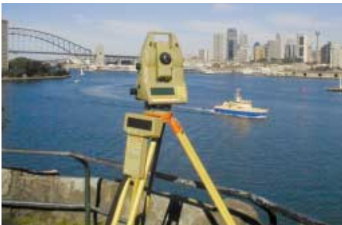
The most comprehensive program of measuring sensors from Leica Geosystems and LH Systems has been used by Peter Noble (PNS) to create a 3D model of North Sydney. Leica Geosystems' TPS and GPS equipment, in conjunction with the RC30 camera, were used to capture the area. Through automated procedures, 1.2 million points were measured and documented, to create one of the most modern city models. This model allows authorities, land owners, utilities and security services to quickly define and analyse every point without leaving the office.
