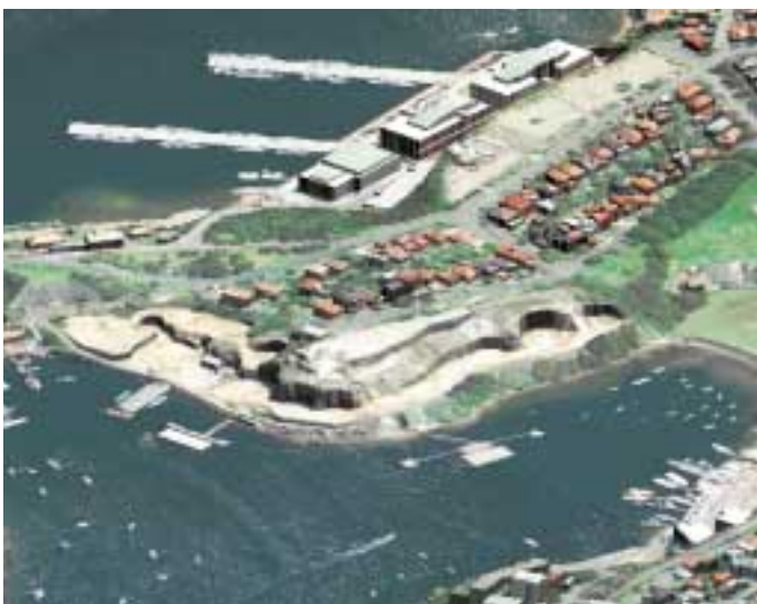
The most comprehensive program of measuring sensors from Leica Geosystems and LH Systems has been used by Peter Noble (PNS) to create a 3D model of North Sydney. Leica Geosystems' TPS and GPS equipment, in conjunction with the RC30 camera, were used to capture the area. Through automated procedures, 1.2 million points were measured and documented, to create one of the most modern city models. This model allows authorities, land owners, utilities and security services to quickly define and analyse every point without leaving the office.
