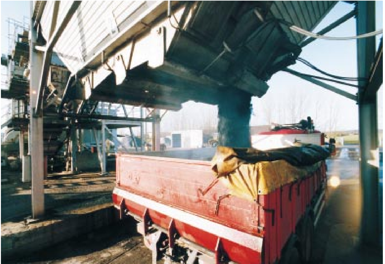
Collection of asphalt from a production plant.
