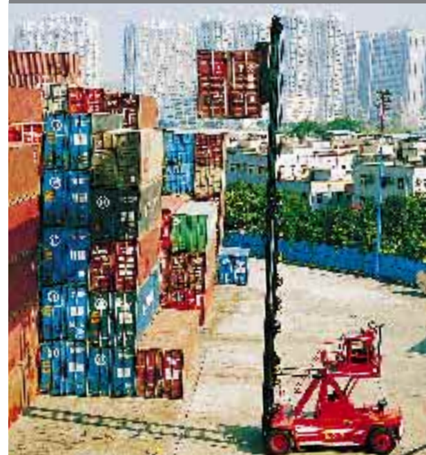
In terminals empty containers are stacked up to 8 containers high.
