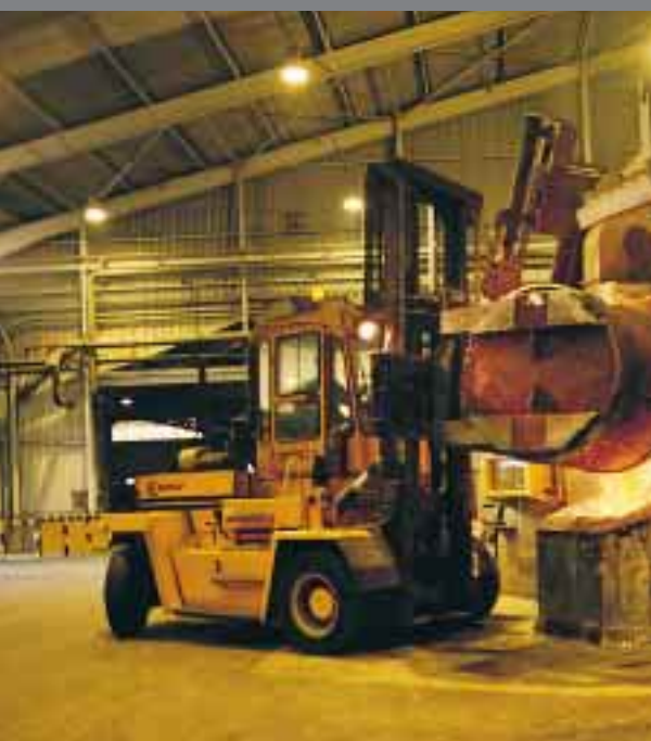
Customised handling solution for the steel industry.
