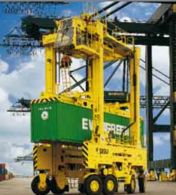
The straddle carrier both lifts, drives and stacks containers.
